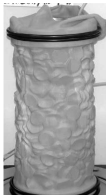
Fig. 2. Specimen made of pure tyre chips.
